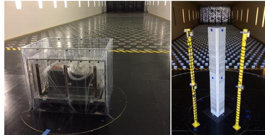
Figure 2. Low-rise pressure tapped model (left) and high-rise aeroelastic model (right).
