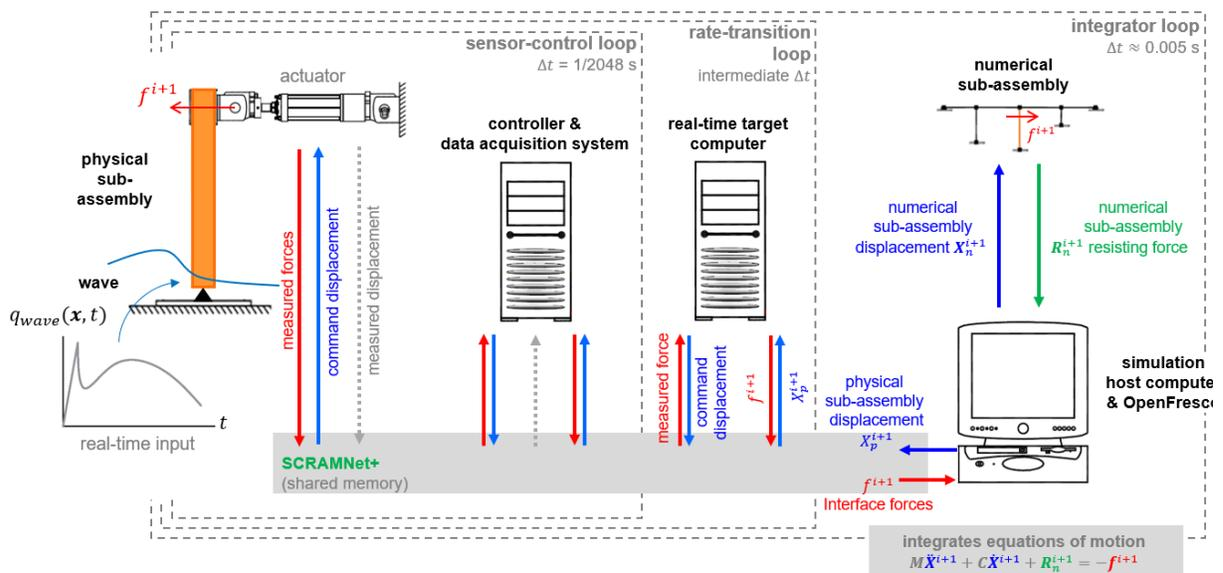
Fig. 6. Hydro-RTHS schematic.
