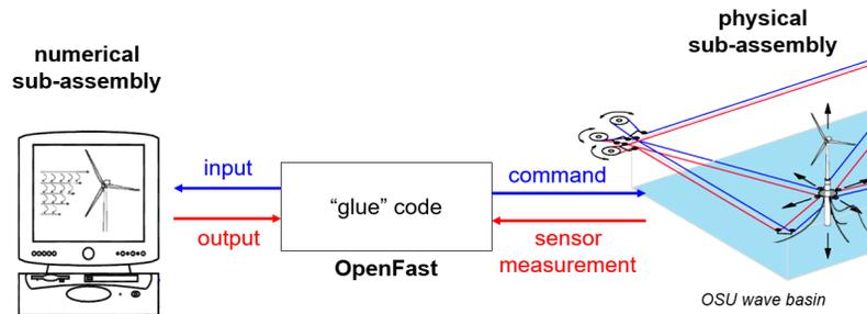
**Fig. 2.** Hydro-RTHS schematic.
