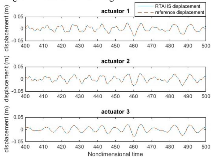
Figure 8. Controlled displacement follows well with reference displacement in RTAHS
