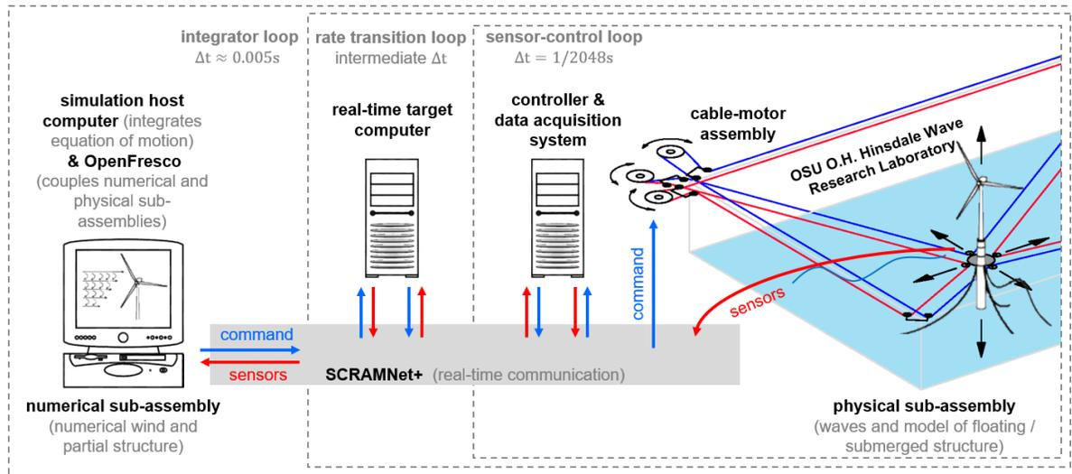
Fig. 3. Hybrid simulation three-tier architecture.
