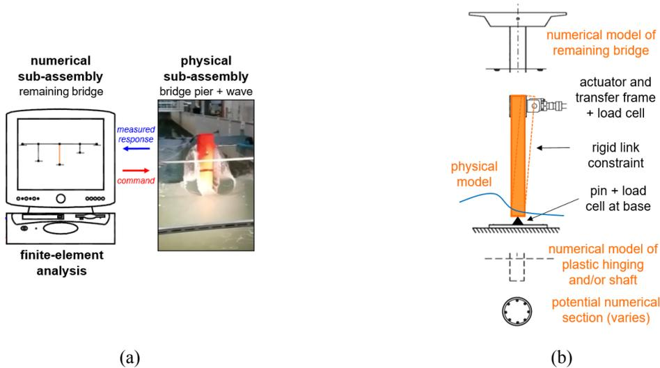
**Fig. 4.** Schematic of hydro-RTHS test: (a) numerical and physical sub-assemblies; (b) numerical model of bridge pier with spring at base to model inelastic response or SFSI effects.
