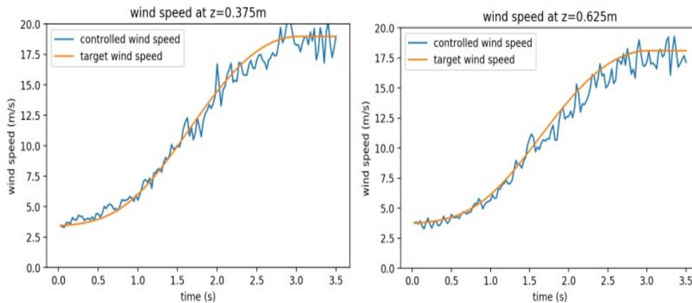
Figure 7. Simulated and target downburst wind fields
