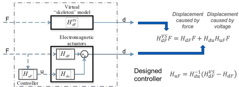
Figure 4. A novel controller design for RTAHS
