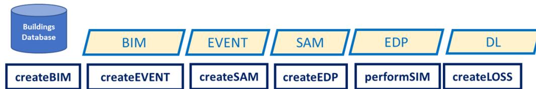
Figure 6-2 Computational workflow and registered applications for the San Francisco Bay Area Earthquake Scenario
