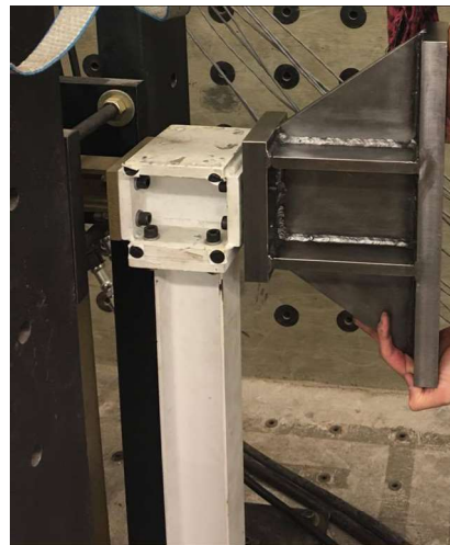
(b) Physical implementation of the coupler attached to the frame
