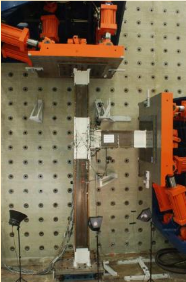
Full-scale slow hybrid simulation for an SMRF beam-column connection
