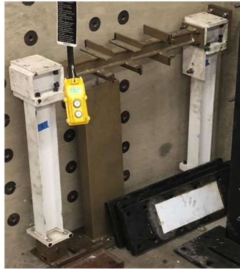
Figure 7: Steel frame comprising the physical substructure: (Left) Drawing (Units: mm), (Right) Photograph.
