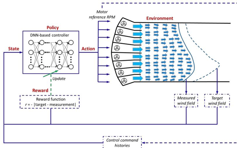
Figure 3. Deep reinforcement learning-based controller for the multiple-fan wind tunnel
