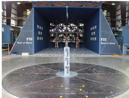
Figure 2: Aerodynamic Testing at the WOW EF
