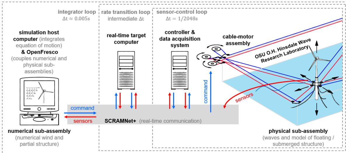
Fig. 3. Hybrid simulation three-tier architecture.
