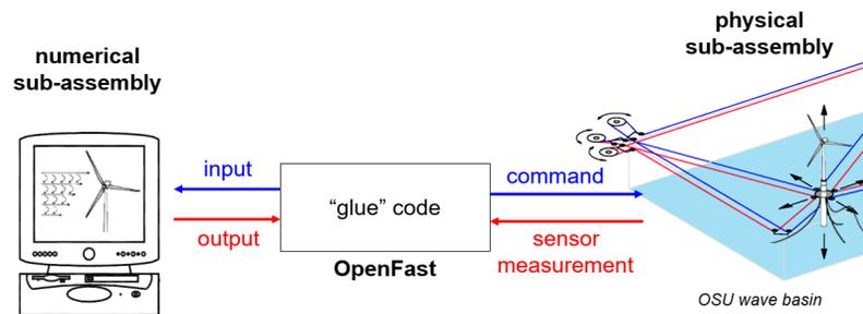
**Fig. 2.** Hydro-RTHS schematic.
