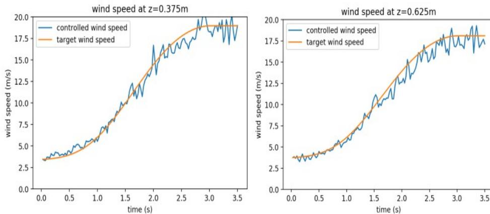
Figure 7. Simulated and target downburst wind fields
