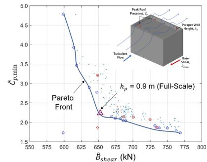
Figure 3. CPS multi-objective optimization of low-rise model.
