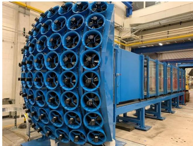
Figure 1. Actively controlled multiple-fan wind tunnel at University at Buffalo
